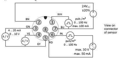
Depending on the value of the connected load resistances  $R_L$ , the analog outputs switch between the operation as voltage interface (0 ... 10 V) and current interface (4 ... 20 mA) automatically.
