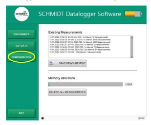
First of all, the data logger settings should be checked or set. For this, click on the *Configuration* button in the left-hand menu column.
