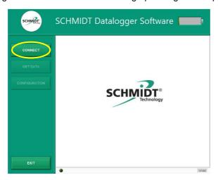
Communication with the data logger is established by clicking the field *Connect* (left column, top).
