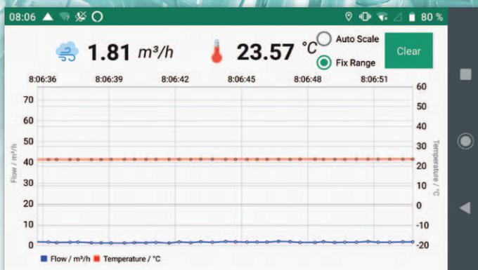
Perfect for use when current measuring values of standard volume flow and medium temperature from different sensors shall be indicated on site temporarily one after another. Important sensor parameters can be customized by the user.
