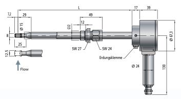
**Remote sensor** including wall mounting bracket
