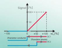
Remark: In an unidirectional design, the switching output OC1 is used as flow indicator by default (configurable). It will clearly show a flow higher than 0 m/s by blocking and will switch if this is less or equal to 0 m/s. Arrows in the representation of the switching outputs mean that the threshold value can be configured. The factory setting for the switching output OC2 is 50% of the measurement range (option: customer-specific switch point).
