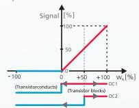
Remark: in an unidirectional design, the switching output OC1 is used as flow indicator by default (configurable). It will clearly show a flow higher than 0 m/s by blocking and will switch if this is less or equal to 0 m/s. Arrows in the representation of the switching outputs mean that the threshold value can be configurated. The factory setting for the switching output OC2 is 50 % of the measurement range (option: customer-specific switch point).
