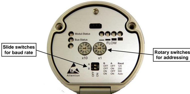
Figure 2 Control elements for manual settings
